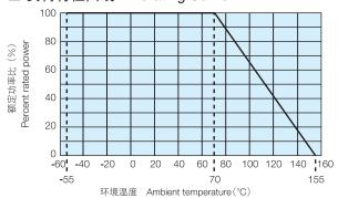
在环境温度 $70^{\circ}$ C以上使用时,应按照上图负荷特性曲线,减小额定功率。 For resistors operated at an ambient temperature of  $70^{\circ}$ C or above, a power rating shall be derated in accordance with the above derating curve.
